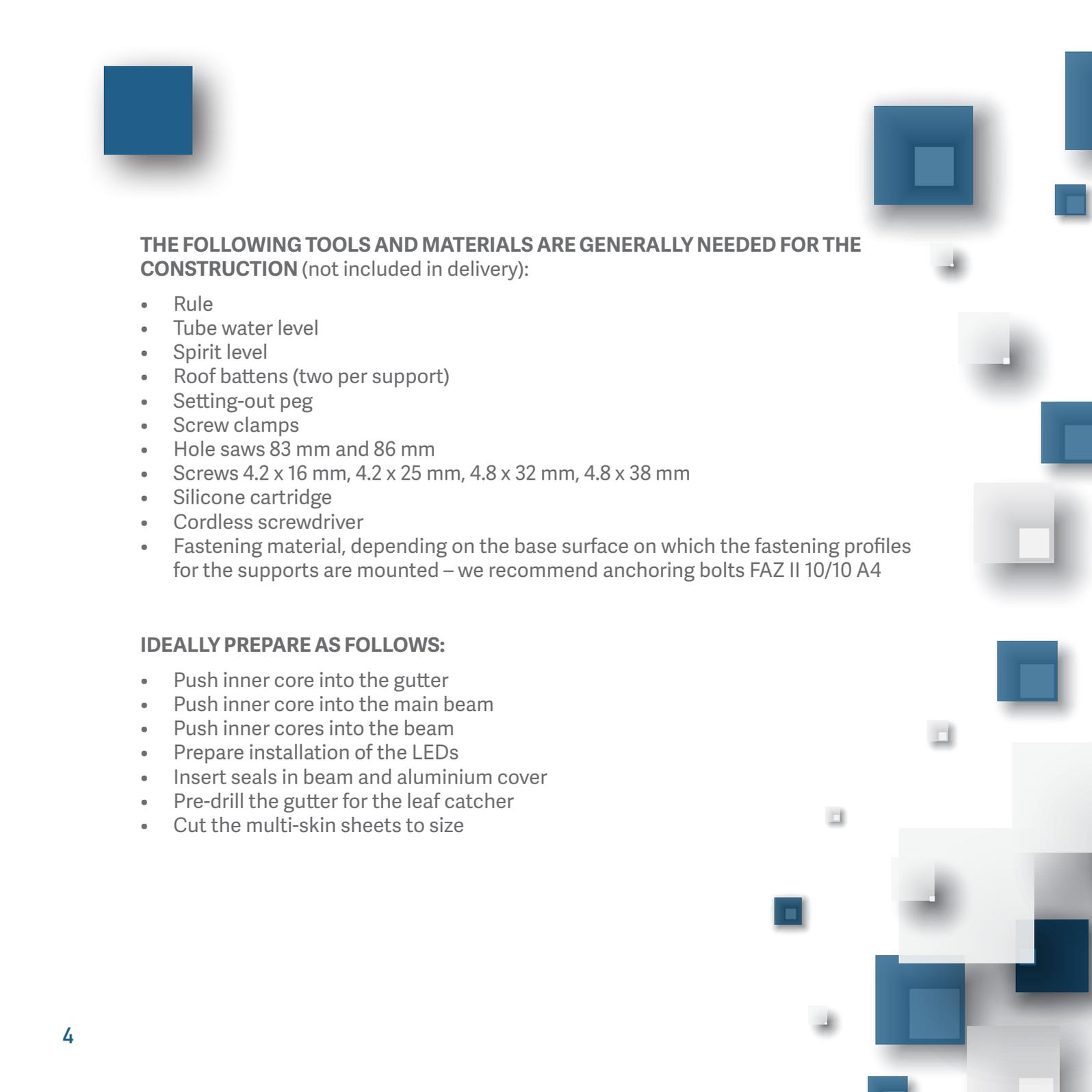
**THE FOLLOWING TOOLS AND MATERIALS ARE GENERALLY NEEDED FOR THE CONSTRUCTION** (not included in delivery):
